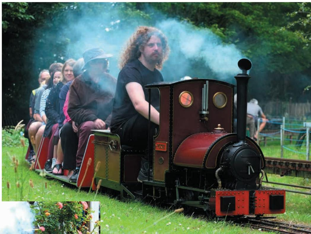
*Pixie* running on the 7.25in gauge line, based on a narrow gauge prototype.
